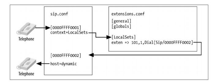
Realize that there actually two different connections being made in an Asterisk system. The first is from the first device to the Asterisk server, the second is from the Asterisk system to the second device. On the part of the first device, the connection has been completed when it connect to the server.
