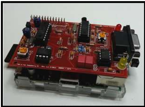
Figure 2: TNC-Pi mounted on a Raspberry Pi
